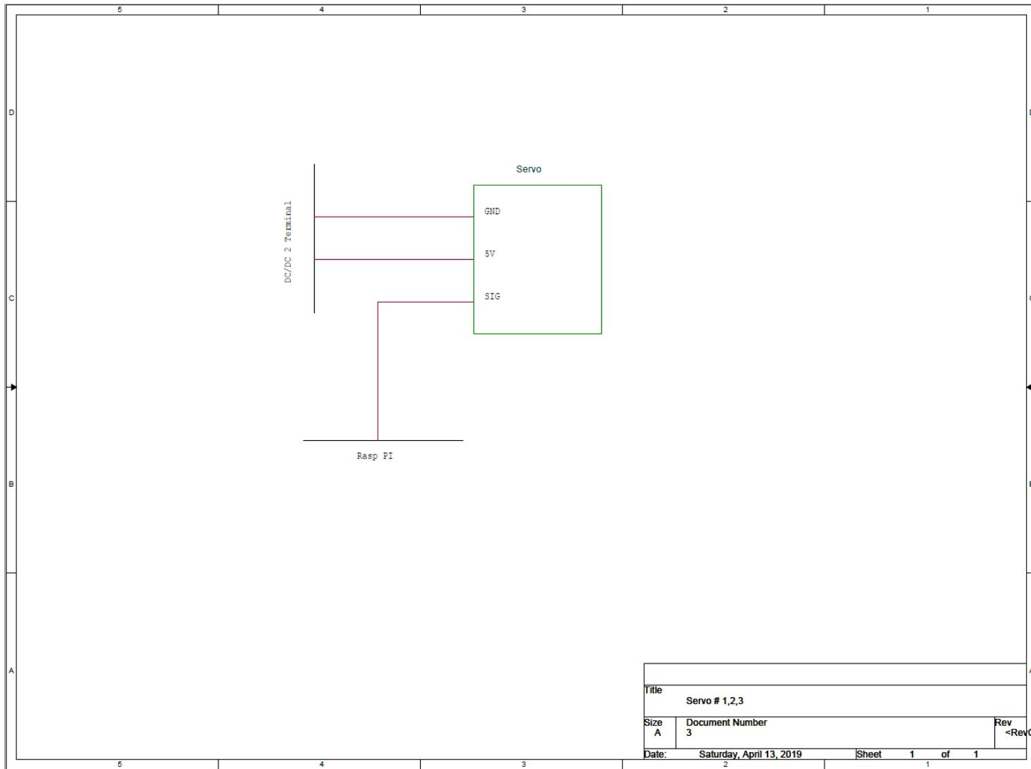
B-9. The robots uses three servos, all three are wired identical. A representation of the wiring is shown in the schematic.
