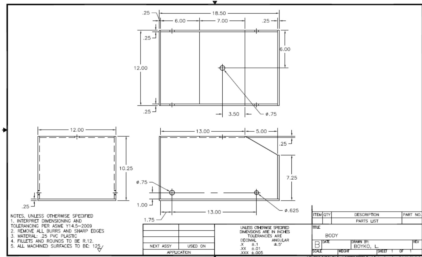
D-1. Mechanical drawing showing the actual body build of the robot.
