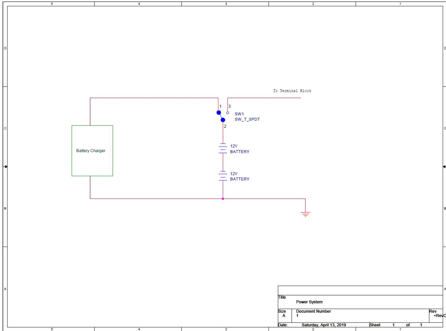
B-7. The schematic represents the wiring diagram of the charging block with a three-way switch to protect the components while in charging mode.
