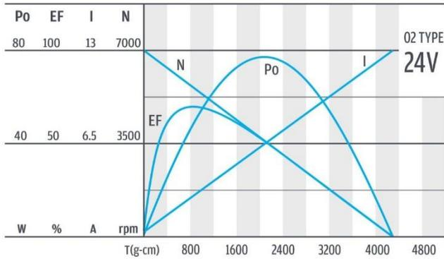
Fig 6. The power, efficiency, current, and rpm over the torque diagram. This is the motor alone without the gear box that we have installed. [28]
